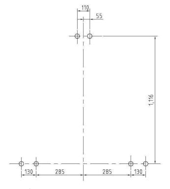
(77-inch Board layout for installation)
